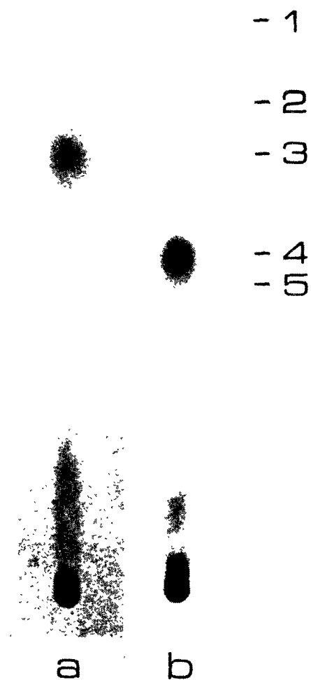
Fig. 1. T.l.c. of methyl ethers of D-[ ^{14}\text{C} ]galactose derived from sialyl- N -acetylactosamine synthesized by: (a) a homogenate of human placenta and (b) a partially purified bovine colostrum enzyme. Radioactivity was detected by autoradiography and reference compounds were detected with aniline phthalate. References were: (1) 2,3,4,6-tetra- O -tetramethyl-D-galactose, (2) 2,3,6-tri- O -methyl-D-galactose, (3) 2,4,6-tri- O -methyl-D-galactose, (4) 2,3,4-tri- O -methyl-D-galactose, and (5) 3,4,6-tri- O -methyl-D-galactose.
